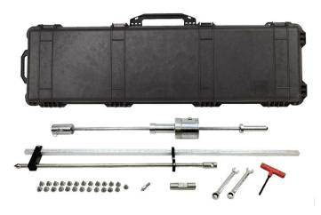
Developed by the Army Corps of Engineers, Dynamic Cone Penetrometers (DCPs) provide a low-cost, efficient test method for quickly determining in-situ CBR values of pavement base, subbase and subgrades. They can readily be used for depths up to 30" and up to 6' with optional drive rods and extensions.
